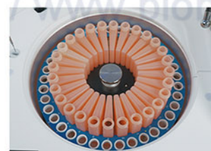
Reagent Tray Refrigerated tray with independent switch.
