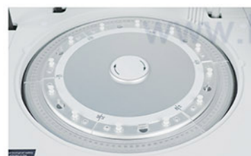
Reaction Tray 37±0.2°C, real-time monitor.
