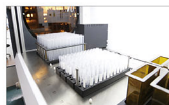
Sample & Reagent & Dilution Rack Module Original sample tubes available; Rack positions programmable.
