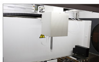
Sample Module Hitech teflon coating probe to prevent cross contamination.
