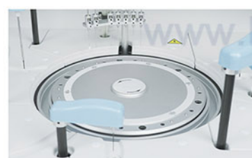
Reaction Tray 37±0.1°C, real-time monitor.
