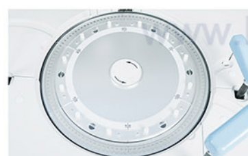
Reaction Tray 37±0.1°C, real-time monitor.
