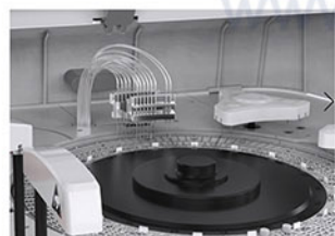
Reaction Tray 37±0.1°C, water bath.
