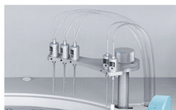
Washing Probe Independent 5-step washing system.
