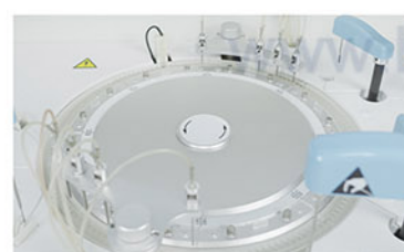
Reaction Tray 37±0.1°C, water bath
