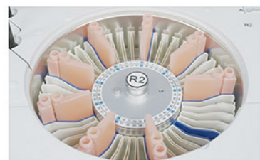
Reagent Tray 2~8°C cooling for 24 hours.
