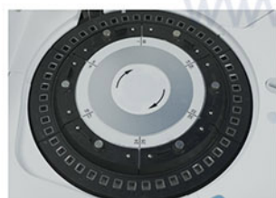
Reaction Tray 37±0.2°C, real-time monitor.
