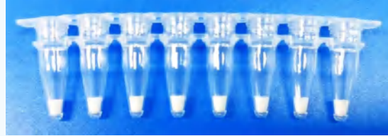
• Figure 2 Morphology of Stool Direct Amplification System after Lyophilized at 55 °C Accelerated for 30 Days.
