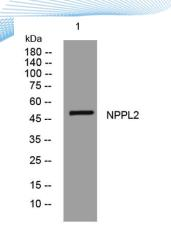
Western blot analysis of lysates from DU145 cells, primary antibody was diluted at 1:1000, 4° over night
