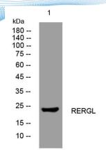
Western blot analysis of lysates from SH-SY5Y cells, primary antibody was diluted at 1:1000, 4° over night
