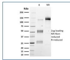
SDS-PAGE analysis of purified, BSA-free Emerin antibody (clone EMD/2167) as confirmation of integrity and purity.
