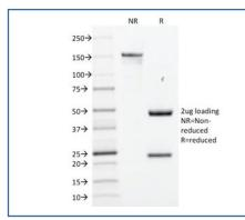
SDS-PAGE Analysis of Purified, BSA-Free SOX-2 Antibody (clone SOX2/1791). Confirmation of Integrity and Purity of the Antibody.
