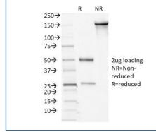
SDS-PAGE analysis of purified, BSA-free Desmocollin 2/3 antibody (clone 7G6) as confirmation of integrity and purity.
