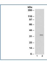
Western blot of HEK293 lysate overexpressing GDF15 probed with GDF15 antibody (mock transfection in lane 1). Predicted molecular weight ~34 kDa.
