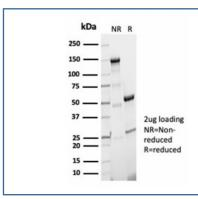
SDS-PAGE analysis of purified, BSA-free recombinant Aciculin antibody (clone PGM5/7005R) as confirmation of integrity and purity.
