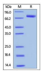
Human SIRP alpha, Mouse IgG1 Fc Tag on SDS-PAGE under reducing (R) condition. The gel was stained with Coomassie Blue. The purity of the protein is greater than 95%.
