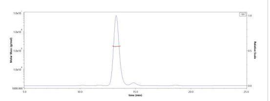
The purity of Human SIRP alpha, Mouse IgG1 Fc Tag (Cat. No. SIA-H52A8) is more than 90% and the molecular weight of this protein is around 140-165 kDa verified by SEC-MALS.
