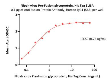
Immobilized Anti-Fusion Protein Antibody, Human IgG1 (5B3) at 1  $\mu$ g/mL (100  $\mu$ L/well) can bind Nipah virus Pre-Fusion glycoprotein, His Tag (Cat. No. FUN-N52H3) with a linear range of 0.1-2  $\mu$ g/mL (QC tested).
